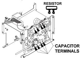
3. Use a DC voltmeter to check that voltage is not present across the terminals on all four capacitors.
